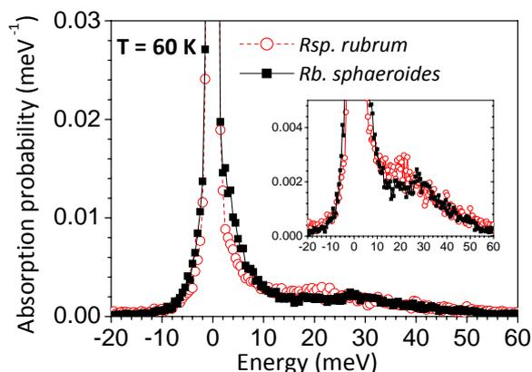
Fig.1. Normalized spectra of nuclear inelastic absorption of synchrotron radiation in the reaction centers from *Rba. sphaeroides* and *Rsp. rubrum*, measured at 60 K. In the inset the absorption probability scale is expanded to show fine differences between the spectra.
