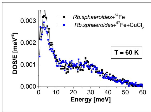
Fig. 4 The density states DOS normalized to their corresponding energies for native and treated with  $\text{CuCl}_2$  *Rb. sphaeroides* measured at 60 K.
