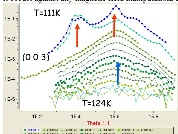
Fig. 3 Temperature dependence of (003) peak in the vicinity of the Verwey transition. Note drastic intensity reduction and two uncorrelated processes marked in red and blue.
