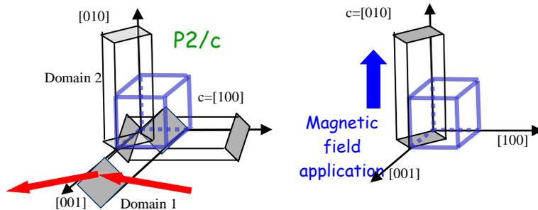
Fig. 1. Experimental layout showing magnetite single crystal (cube) with 3 possible monoclinic domains and the domain 1 inspected by X ray beam. Under external magnetic field only the domain 2 survives, causing essentially no reflections.
