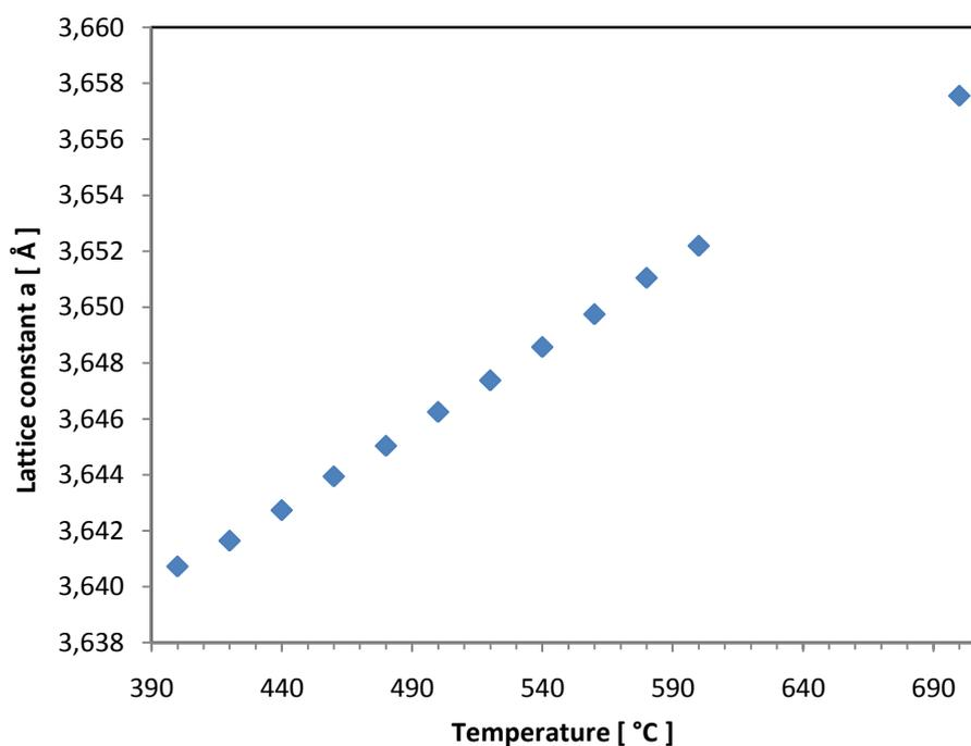
Fig. 1 Temperature dependence of the lattice constant  $a$  for  $\text{CaCu}_3\text{Ti}_4\text{O}_{12}$ .
