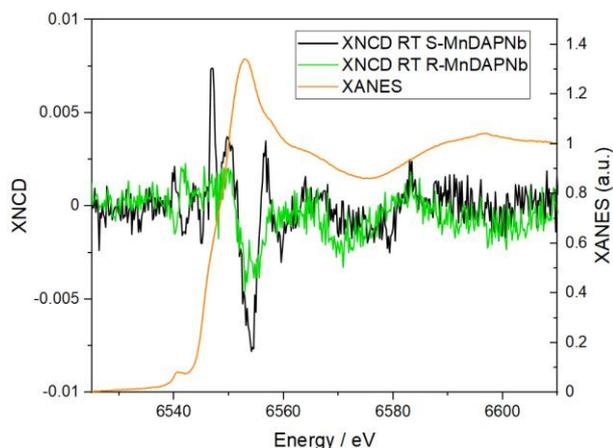
Figure 1. Two XNCD signals (at 6540 eV and at 6542 eV) for *S*- and *R*-MnDAPNb crystals at room temperature. Stronger signals on the graph does not change sign with enantiomer, they may be the result of decomposition of sample or diffraction peaks.
