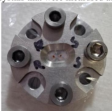
Figure 2. Holder for low temperature measurements in magnetic field with crystals *S*- and *R*-MnDAPNb.
